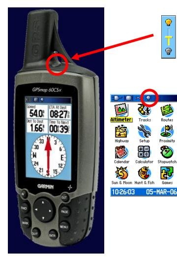
To minimize battery drain, limit or turn off backlight Press and quickly release the POWER button. Press up on ROCKER to increase, down to decrease. Press ENTER or QUIT to close **Backlight adjustment** window.
